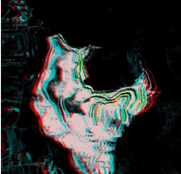
Figure 4: The ALOS stereomodel for the Markopoulo open-pit limestone mine. The black line shows the digitized head of the planes and the green shows the foot. The figure can be seen in 3D using Red & Green-Blue glasses.
