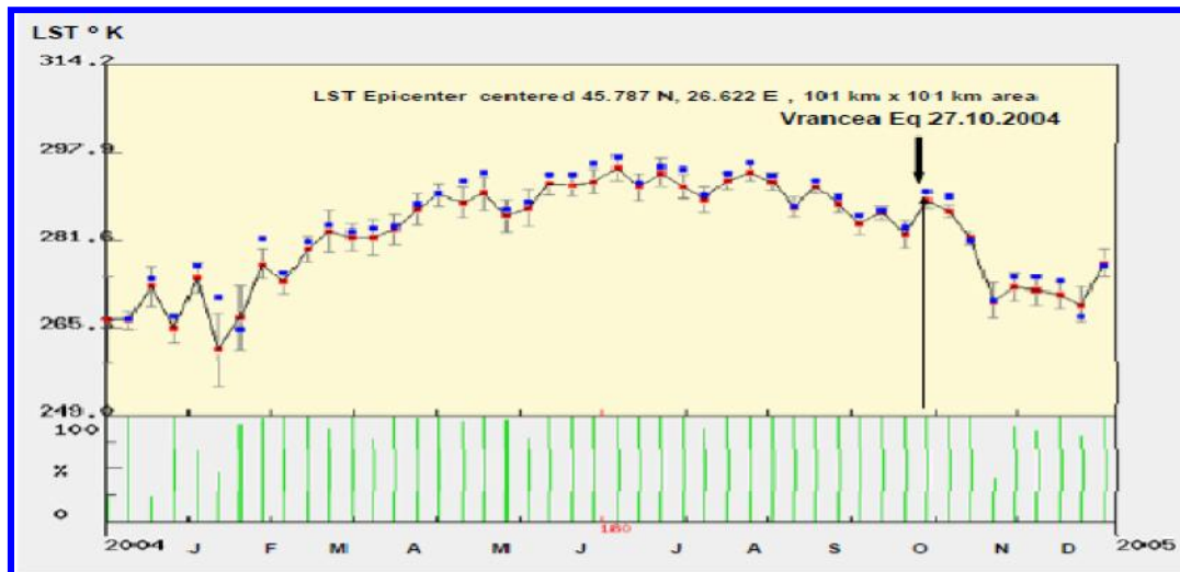
Figure 2. Land surface temperature (LST) variation during 2004 year over epicentral Vrancea region based on MODIS Terra time series data.
