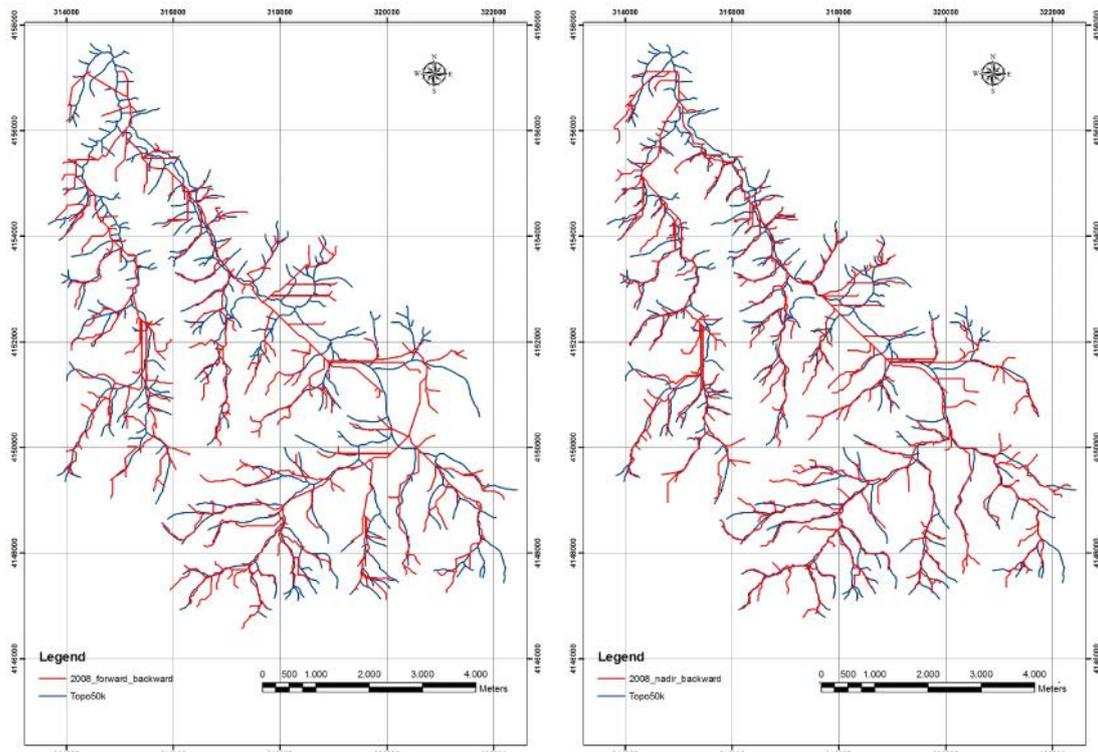
Figure 1: At the left: The extracted drainage network from the ALOS 2008 forward-backward stereo pair. At the right the extracted drainage network from the ALOS 2008 nadir-backward stereo pair. The reference network from the topographic maps is presented with blue colour.
